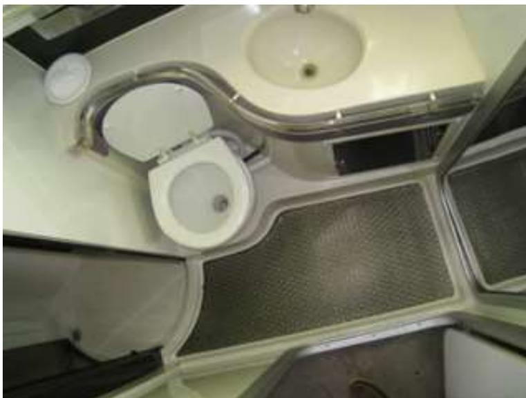
The head is in very good condition. The head is equipped with shower, hand basin and an electric marine standard toilet. The shower unit is an integral part of the inner liner. The shower stall is good sized fiberglass enclosure. The shower is equipped with a sump pump and overboard drain. There is a macerator unit, Y-gate, and holding tank installed. The head plumbing is in good condition and conforms to A.B.Y.C. standards.
