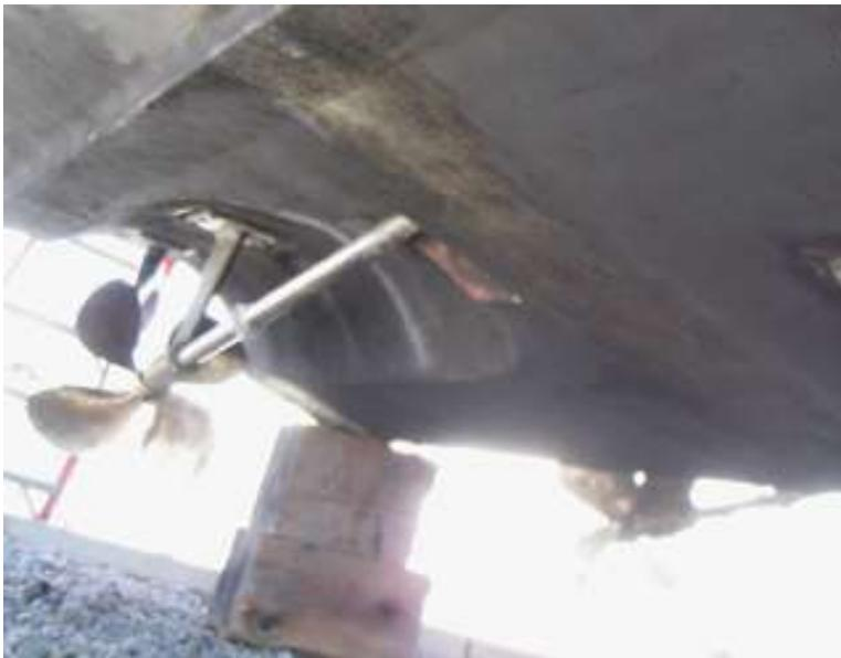
The hull is a typical polyester laminate reinforced with fiberglass matt and woven roving in a modified deep Vee configuration. The freeboard finish is white gelcoat with stainless trim, and is in very good condition, overall, with just a few superficial mars and scratches.
