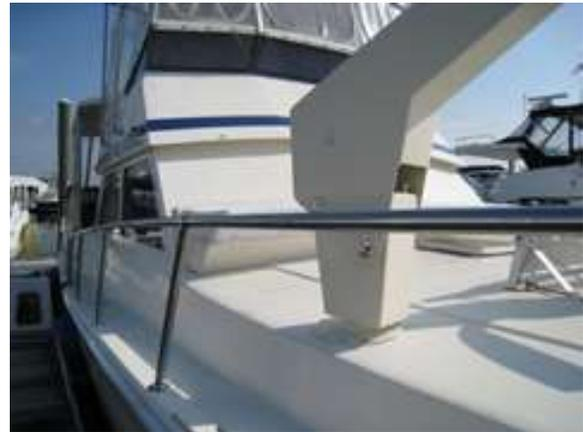
area. The canvas enclosure, and supporting structure appear to be a recent upgrade. The bridge is equipped with stainless life rails which are secure and properly backed. Overall, the bridge, including the operating station and upholstery is in excellent condition. The top of the bridge is solid fiberglass and well secured and sturdy.
