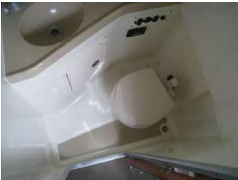
The head is a multi piece fiberglass enclosure which forms part of the inner liner. It is properly secured to the hull and forms an integral part of the hull unit. It houses a VaccuFlush - electric toilet, hand wash basin, and shower gear. The head
