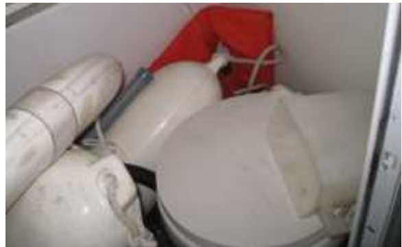
Head with toilet and macerator with holding tank has never been used.
