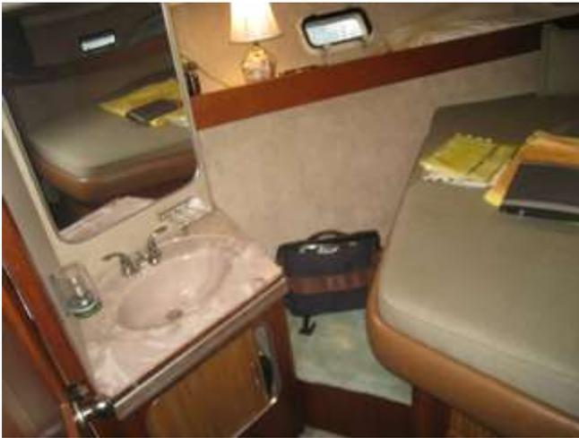
The head liners in both areas are clean and in good condition and secure. All escape hatches are in working condition and tight to the weather.
