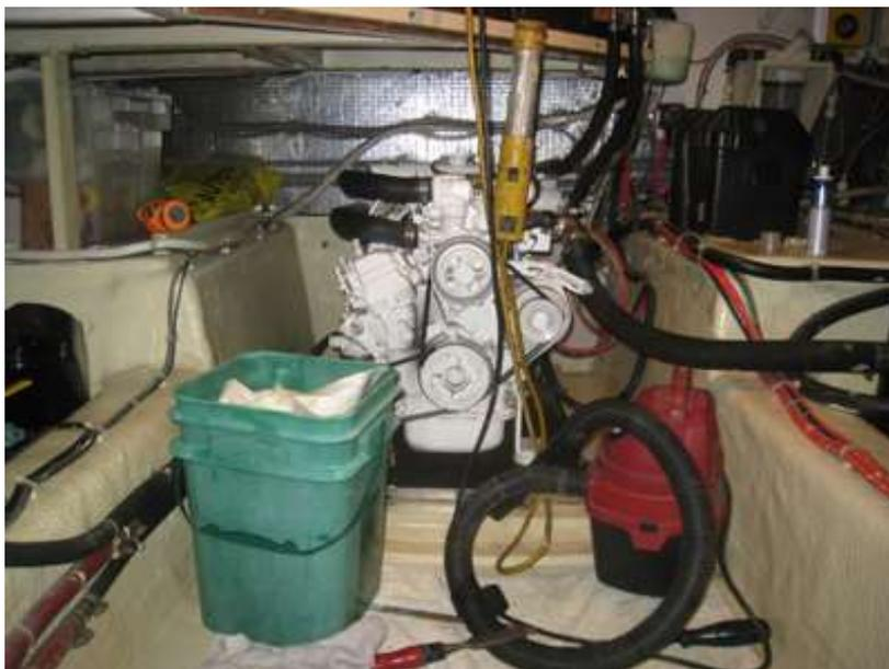
The bilge in this area is in good shape. There are adequate bilge pumps installed and working in this area. There is no oil in the bilge. The raw water intakes are equipped with a proper sea water strainers, and are secure.
