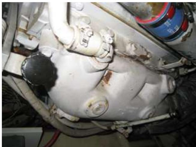
The exhaust system is cast and rubber, with fiberglass silencers, heavy duty, and appear to be recent upgrades. All exhaust hoses and related connections are secure. The system clamps are all doubled and in good shape.
