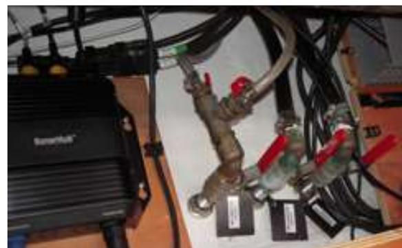
approved type and properly installed and grounded. There is a proper sea water strainer installed just aft of the engine cooling intake.
