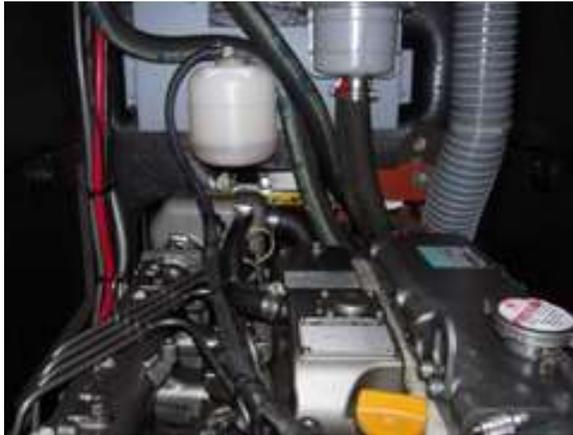
engine compartment bilge is epoxy painted, sound and sturdy. The bilge in this area is clean. There are adequate bilge pumps installed and working in this area. There is no oil in the bilge. All fuel and water tanks are in good condition as can be inspected. The fuel lines, including a Racor filter are approved type and in good condition. The flex fuel line appears to be a recent upgrade. The fuel fills, vents and shut-off are in good order. The EM 2000 engine monitor is a recent upgrade.
