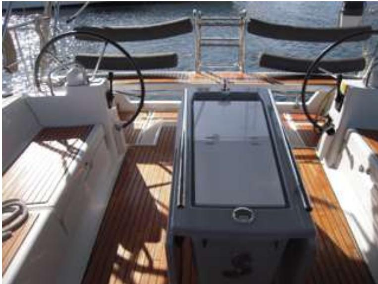
The topsides are well secured, and are in good condition with no abrasions or damage. No soft spots were noted on the deck. All outside wood surfaces and trim are teak and in very good condition. The bow and stern pulpits and life line stanchions are constructed of stainless steel and properly secured and backed. The life lines and
