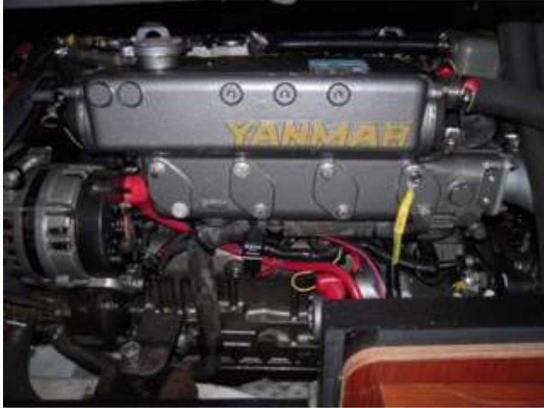
Propulsion is by a 57 HP fresh water cooled Yanmar diesel engine with Yanmar Sail Drive reduction gear.
