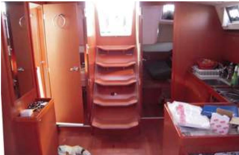
Photo at left is a view of the companionway entry ladder to the main cabin, The entire unit folds upward for easy access to the engine compartment.
