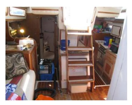
Lighting is good throughout the vessel. The dinette table is large and properly secured to the structure. There is adequate locker and drawer space in the main cabin. There is hanging locker and cabinet space between the main cabin and the v-berth. These interior areas, overall, appear in good, solid condition.
