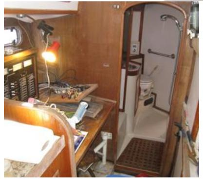
The main AC/DC panel is properly grounded and all AC circuits are properly protected but not isolated from the DC side. A new isolation transformer should be installed as well as a complete bonding system. The AC circuits were not checked out while operating.
