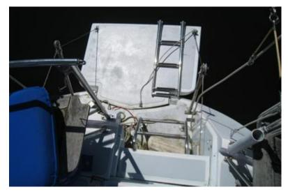
The dinghy lift system is secure. The cockpit (rigid) screen is well secured to the cockpit coaming and is in good condition. The steering pedestal and attachments are secure. The jib sheet tracks are in good shape and secure. The companionway hatch is in good condition. The vertical section of the hatch fits nicely and is secure. All mooring cleats are secure. Overall, the foredeck and cockpit are in very good condition.
