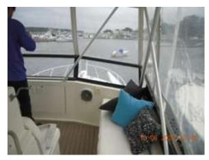
area. The canvas enclosure, and supporting structure appear to be a recent upgrade. The bridge is equipped with stainless life rails which are secure and properly backed. Overall, the bridge, including the operating station and upholstery is in excellent condition. The top of the bridge is solid fiberglass and well secured and sturdy.
