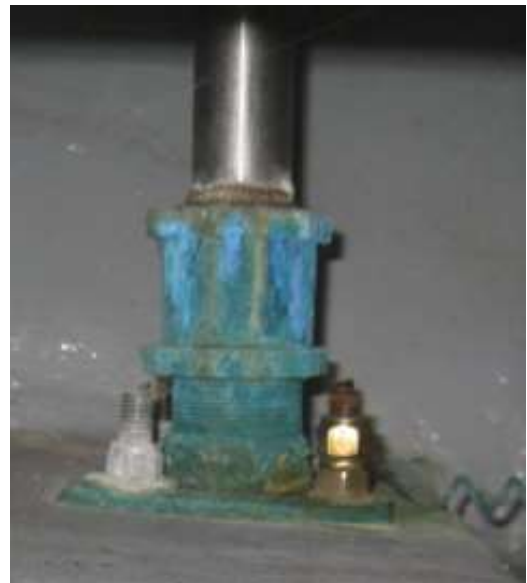
Port rudder shaft log is leaking, needs service
