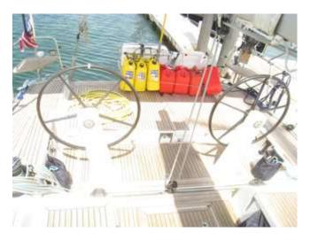
The wheels, (there are two after market Kevlar), pedestals, quadrant, cables, and all related steering gear are in excellent well maintained condition and working properly. There is a provision for an emergency tiller, and the tiller was on board.
