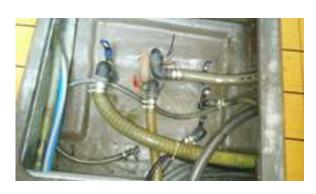
cables are smooth operating. The engine compartment bilge is epoxy painted, sound and sturdy. The bilge in this area is clean. There are adequate bilge pumps installed and working in this area. There is no oil in the bilge. All fuel and water tanks are in good condition as can be inspected. The fuel lines, including a Racor filter are approved type and in good condition. The flex fuel line appears to be a recent upgrade. The fuel fills, vents and shutoff are in good order.
