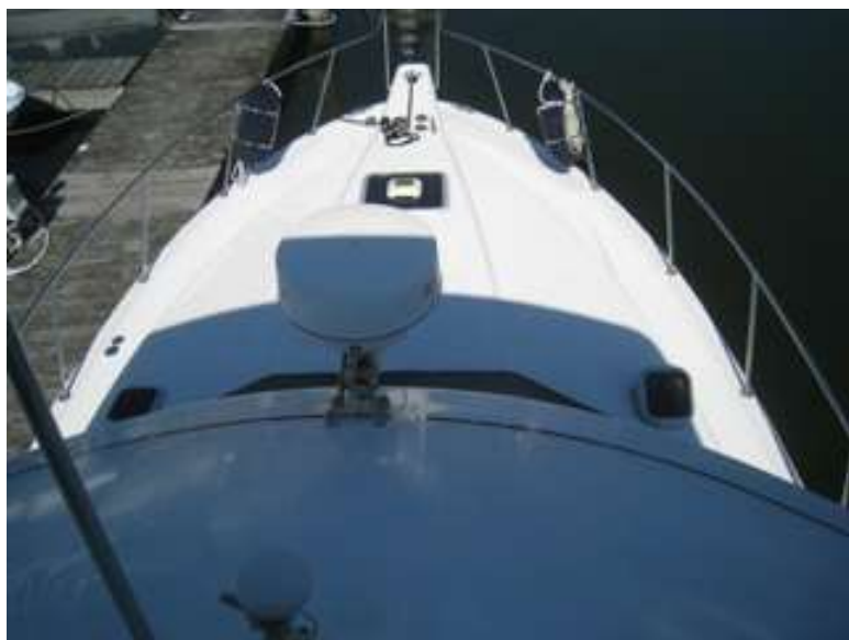
View of bow deck, life rail and anchor pulpit
