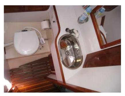
The head is also a multi piece laminate enclosure with built in shower. It is properly secured to the hull and forms an integral part of the hull unit. It houses a vanity with hand basin, manual flush marine toilet and shower. The shower pump out device is in good, clean condition. There is a macerator unit installed. This unit appears in good condition.
