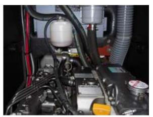
engine compartment bilge is epoxy painted, sound and sturdy. The bilge in this area is clean. There are adequate bilge pumps installed and working in this area. There is no oil in the bilge. All fuel and water tanks are in good condition as can be inspected. The fuel lines, including a Racor filter are approved type and in good condition. The flex fuel line appears to be a recent upgrade. The fuel fills, vents and shut-off are in good order. The EM 2000 engine monitor is a recent upgrade.
