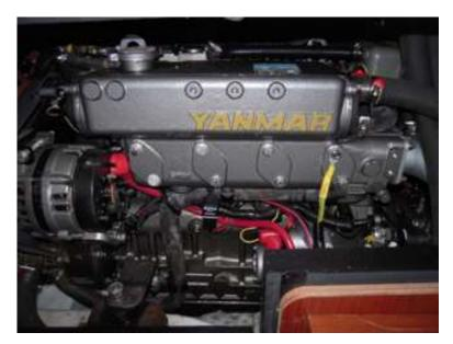
Propulsion is by a 57 HP fresh water cooled Yanmar diesel engine with Yanmar Sail Drive reduction gear.
