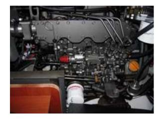
The gen set is an Onan Cummins Diesel powered 7.5 KW and is in good shape. The bow thruster and related hardware appear lightly used. The wiring and connections to the thruster are of the appropriate size and are secure.
